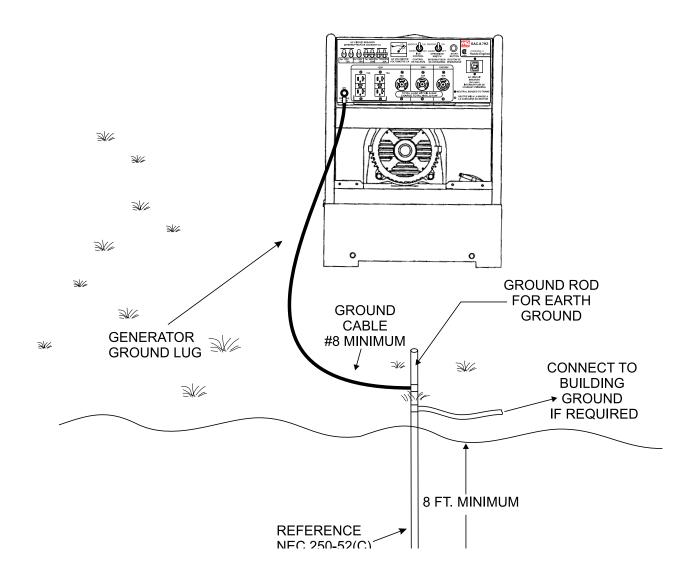
Figure 2. Generator Grounding
